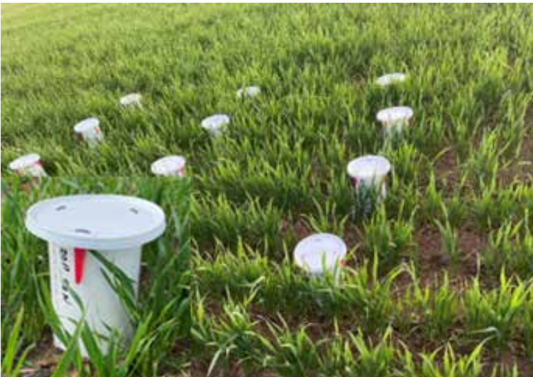
Chambers for ammonia gas measurement in the field
